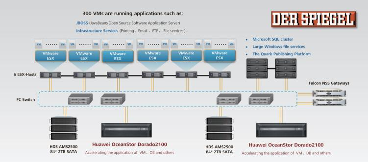
Huawei worked closely with Der Spiegel to design and implement a SSD storage system that fulfills these requirements. The result was the implementation of 2 Huawei Dorado2100 SSD Storage systems, each containing 24 SSD disks with a capacity of 100GB per disk. The total storage capacity for each Dorado2100 is 2.4TB, resulting in an overall capacity of 4.8TB.
